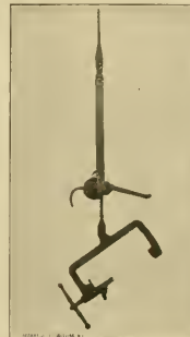
DEVICE FOR HOLDING DRAWBAR WHILE YOKES ARE BEING RIVETED ON
